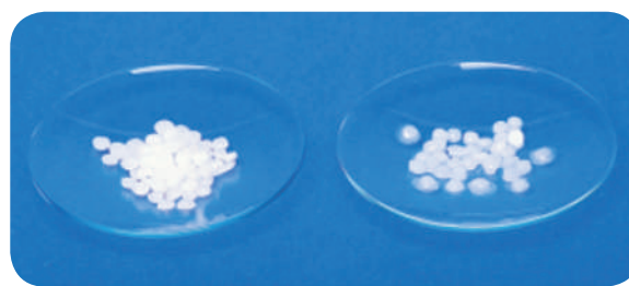
Figure 9.11 Deliquescence in Sodium hydroxide
