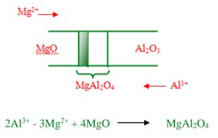
2) At interface of MgAl<sub>2</sub>O<sub>4</sub>/Al<sub>2</sub>O<sub>3</sub>
