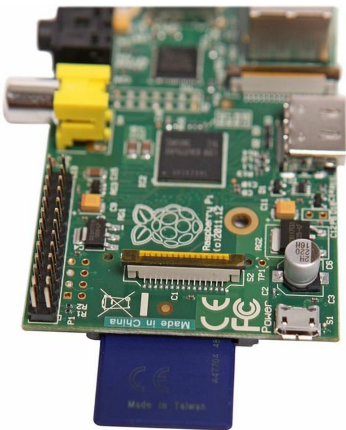
FIGURE 1.7 A properly seated SD card.
