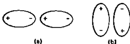
Fig. 8.4 (a) Head-to-tail arrangement of dipoles; (b) antiparallel arrangement of dipoles.
